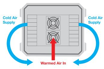
Typical TEU setup looking towards air conditioning unit indicating cold and warm airflow
