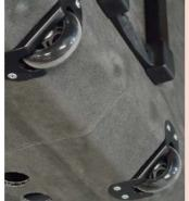
Test results of 34.5kg drop from 500mm Test 1 – On Wheels Test 2 – On Side Test 3 – On Front
