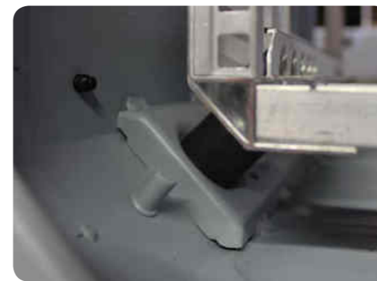
Internal CV2 chassis with elastomeric AVM and welded anchor plate
