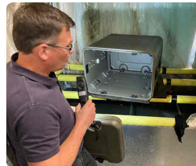
Internal inspection after water test
